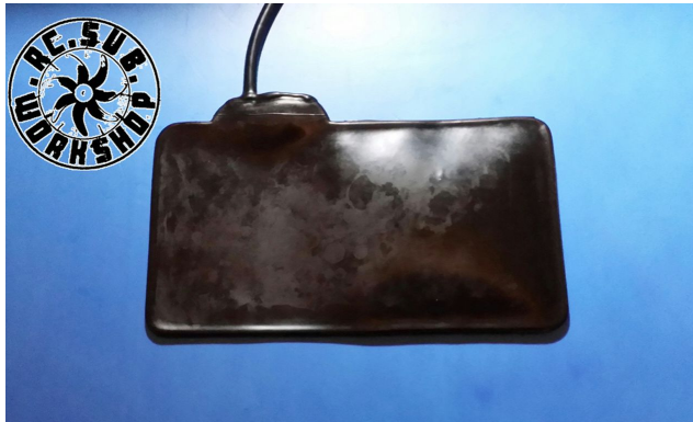
Figure 5.3.1: Bladder ballast system
